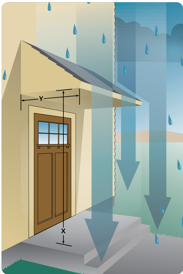
X= Distance from bottom of door. Y= The amount of overhang protection required.
